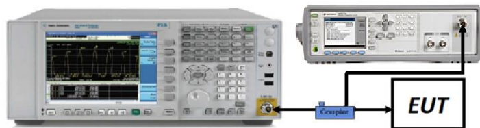
Figure 7-1. Test Instrument & Measurement Setup
