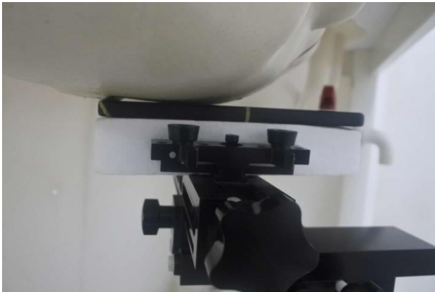
Right Cheek, Test Separation 0 mm
