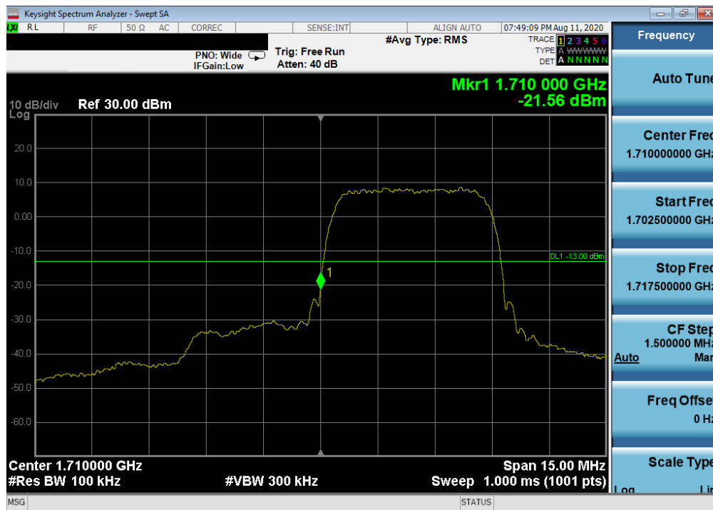
Plot 7-72. Lower Band Edge Plot (WCDMA AWS – Ch. 1312)
