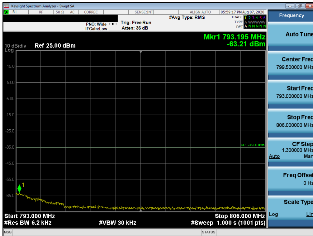
Plot 7-67. Upper Emission Mask Plot (LTE Band 13 - 10MHz QPSK – Full RB Configuration)
