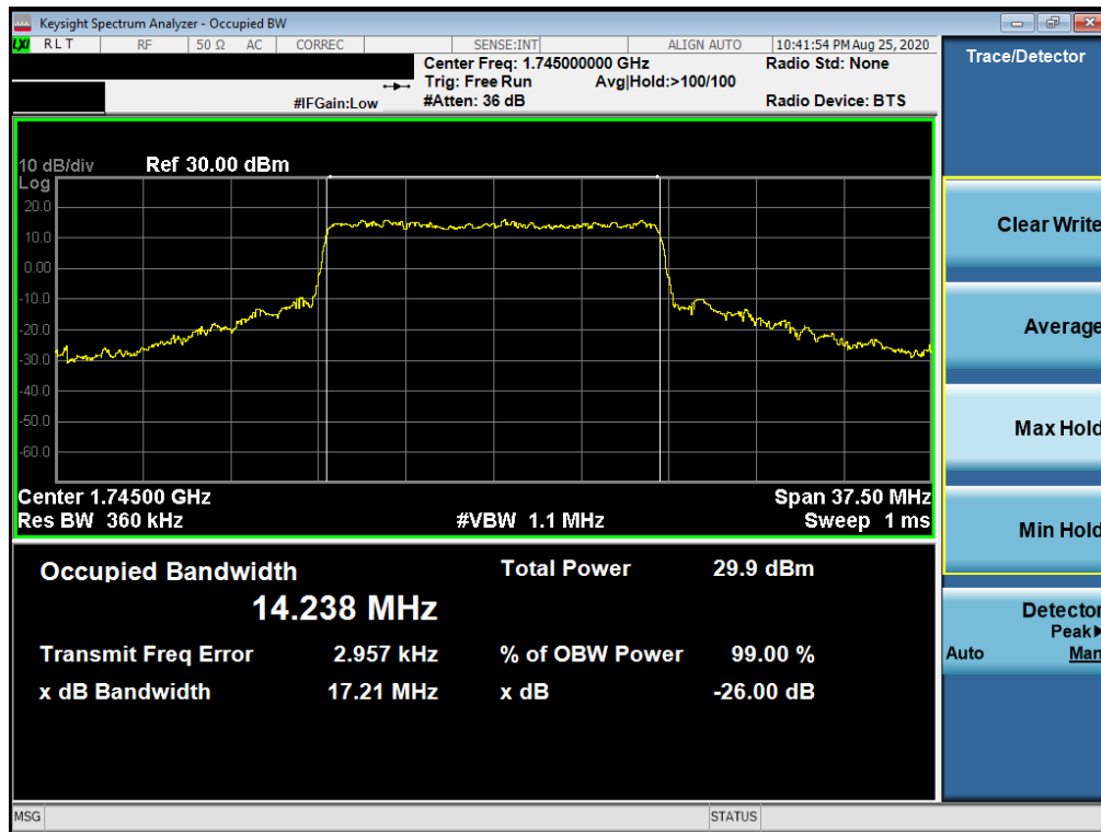
Plot 7-45. Occupied Bandwidth Plot (NR Band n66 - 15.0MHz CP-OFDM 64QAM - Full RB)
