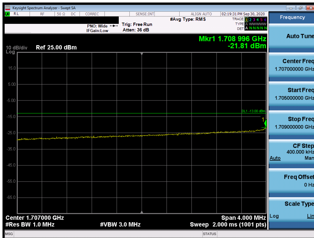
Plot 7-89. Lower Extended Band Edge Plot (LTE Band 66/4 - 10MHz QPSK – Full RB Configuration)
