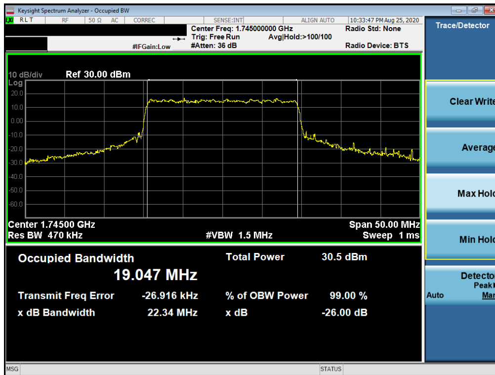
Plot 7-40. Occupied Bandwidth Plot (NR Band n66 - 20.0MHz CP-OFDM 16QAM - Full RB)
