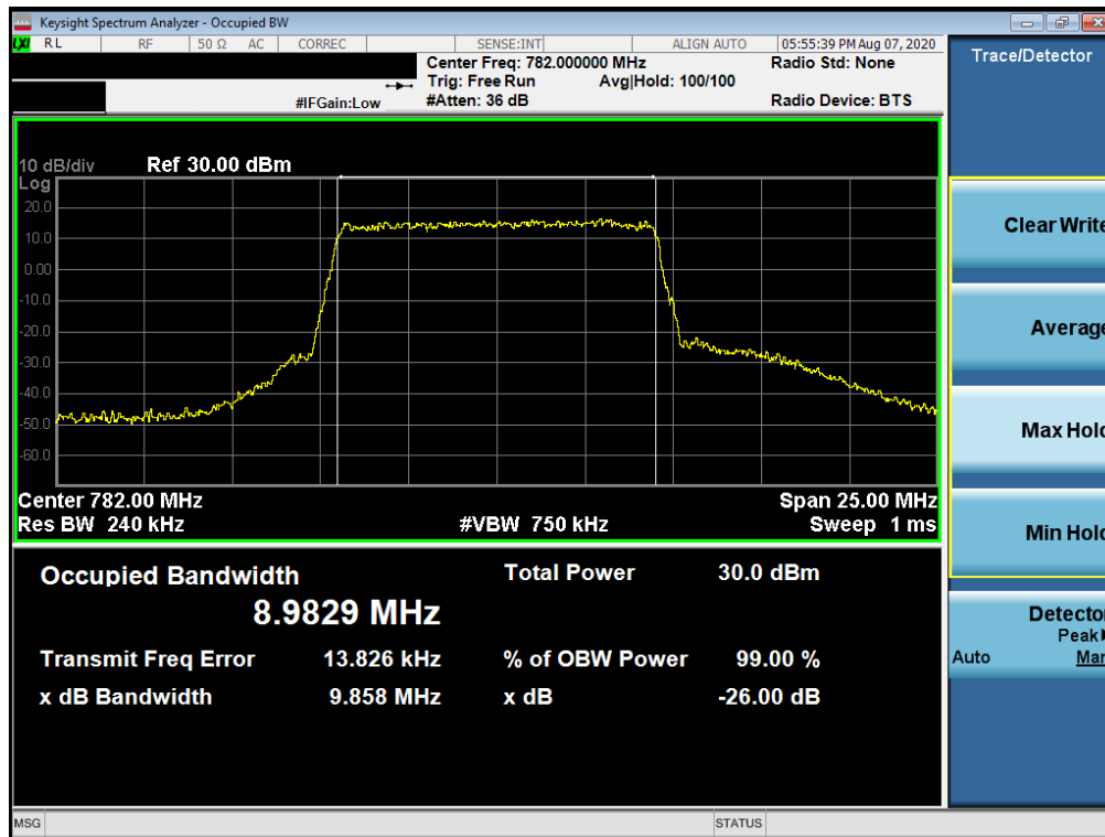
Plot 7-15. Occupied Bandwidth Plot (LTE Band 13 - 10MHz 64-QAM - Full RB Configuration)
