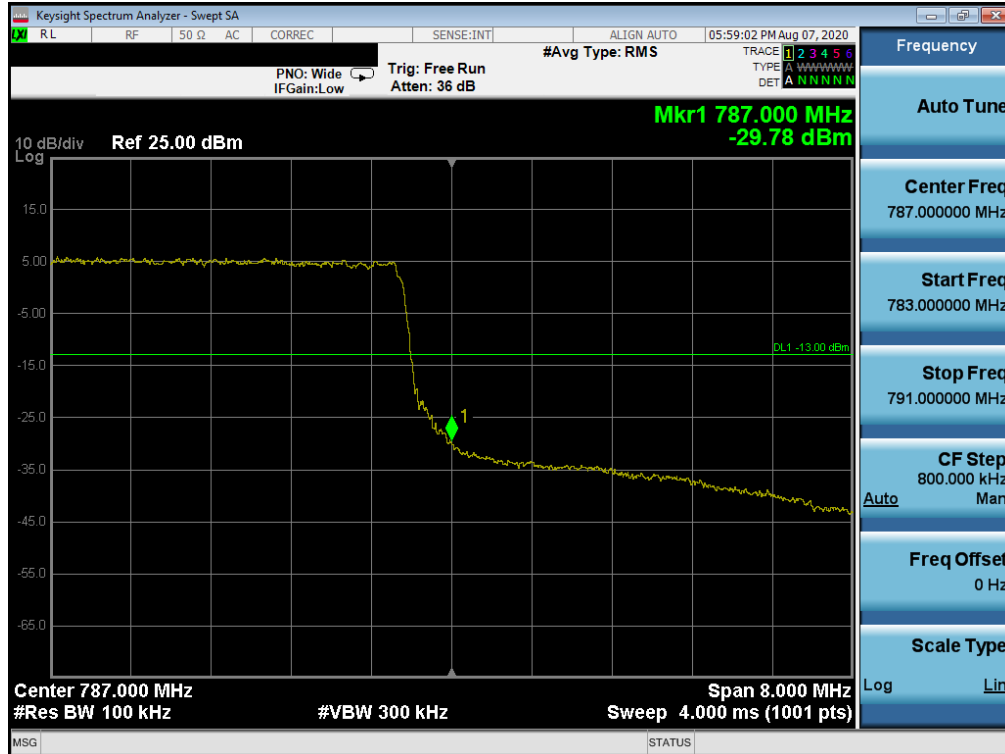
Plot 7-66. Upper Band Edge Plot (LTE Band 13 - 10MHz QPSK – Full RB Configuration)
