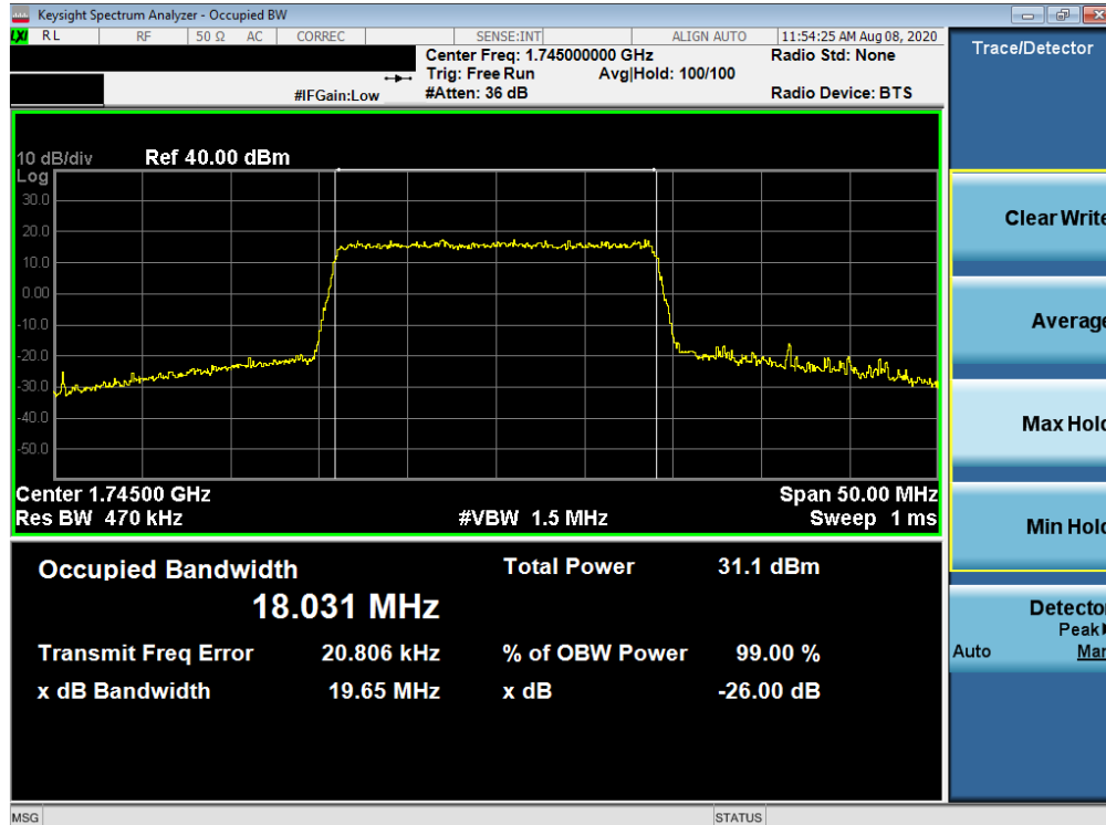
Plot 7-21. Occupied Bandwidth Plot (LTE Band 66/4 - 20MHz 16-QAM - Full RB Configuration)
