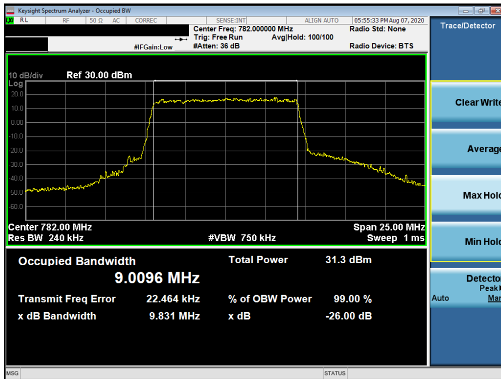
Plot 7-14. Occupied Bandwidth Plot (LTE Band 13 - 10MHz 16-QAM - Full RB Configuration)
