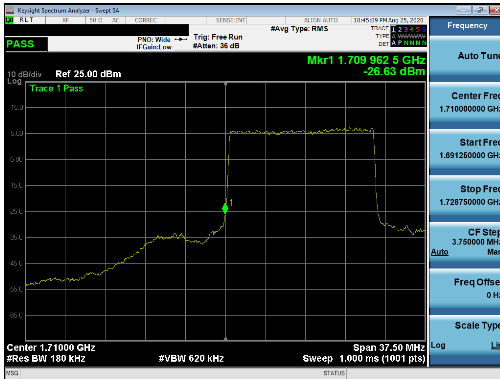
Plot 7-116. Lower Band Edge Plot (NR Band n66 – 15.0MHz - Full RB)
