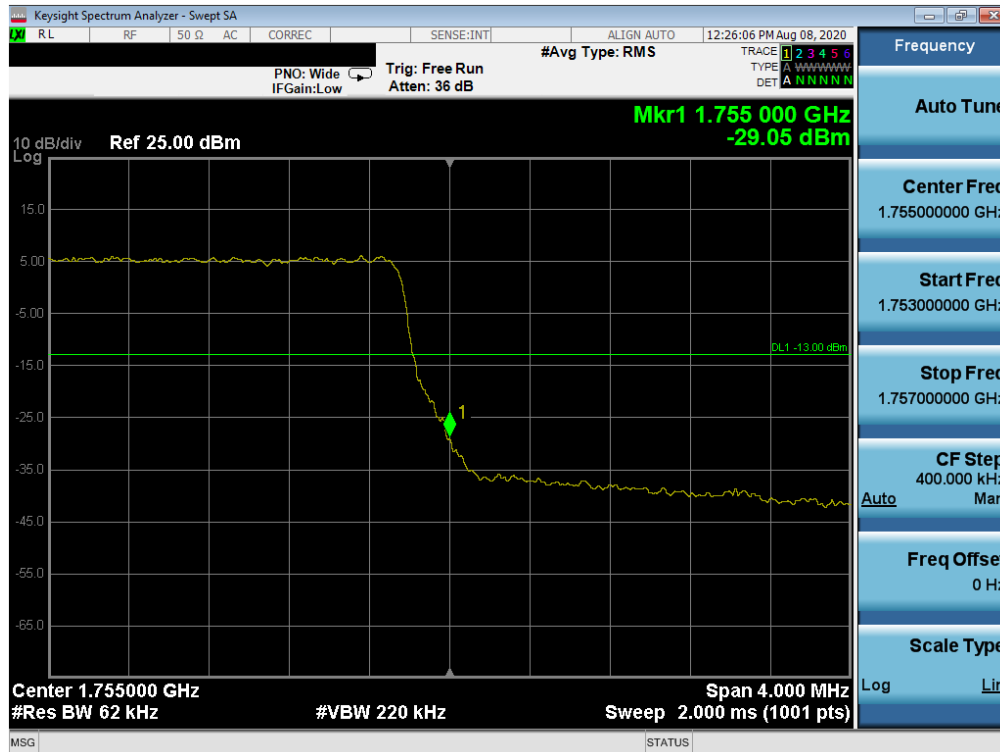
Plot 7-96. Upper Band Edge Plot (LTE Band 4 - 5MHz QPSK – Full RB Configuration)
