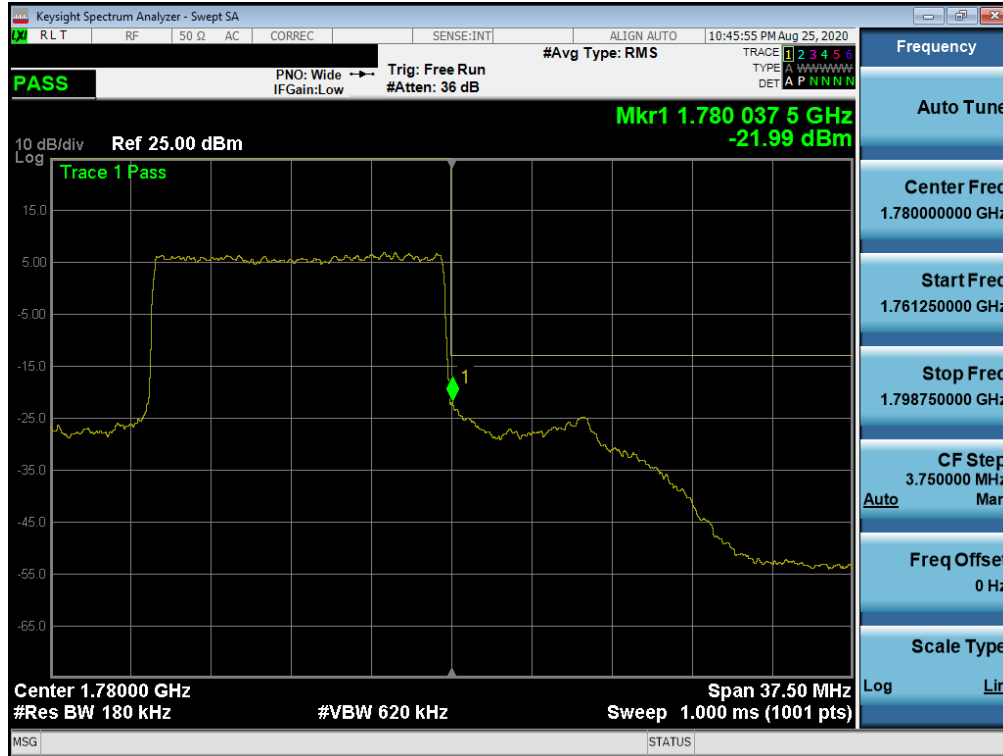
Plot 7-118. Upper Band Edge Plot (NR Band n66 – 15.0MHz - Full RB)
