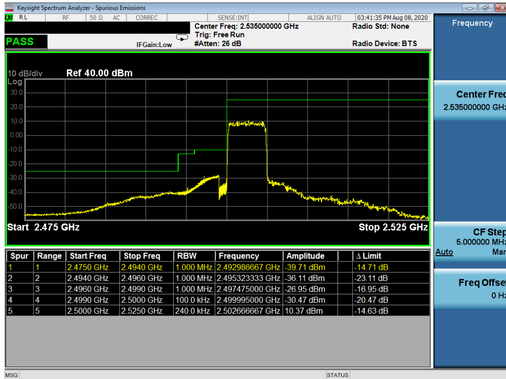
Plot 7-49. Lower ACP Plot (LTE Band 7 - 5MHz QPSK – Full RB Configuration)
