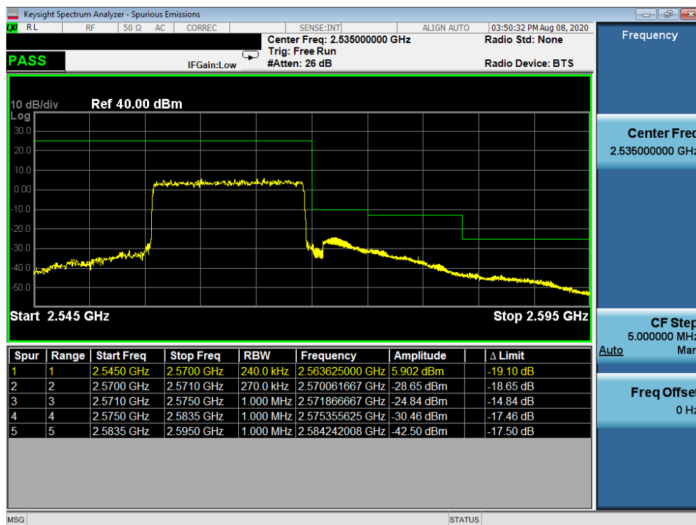
Plot 7-46. Upper ACP Plot (LTE Band 7 - 15MHz QPSK – Full RB Configuration)
