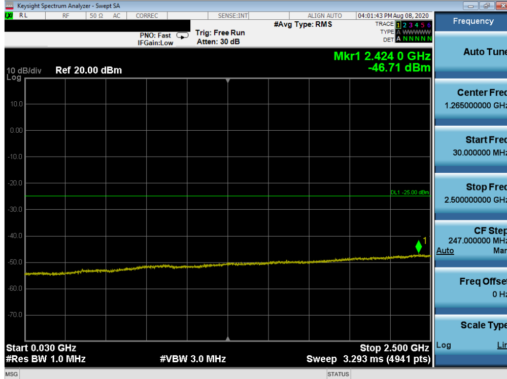
Plot 7-31. Conducted Spurious Plot (LTE Band 7 - 20MHz QPSK - RB Size 1, RB Offset 0 - High Channel)
