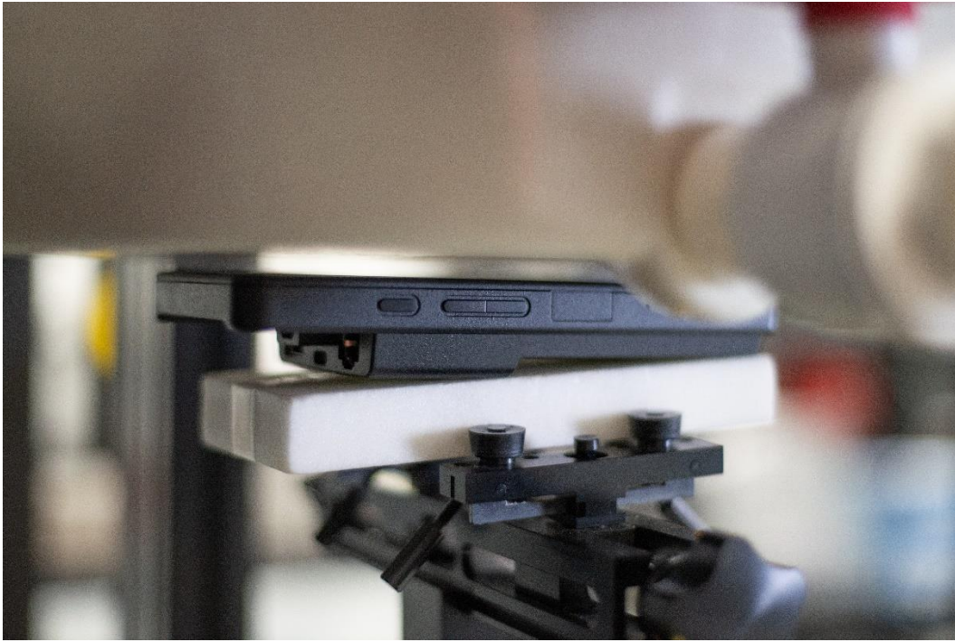
Figure C SAR Test Setup – Body – Front 5mm
