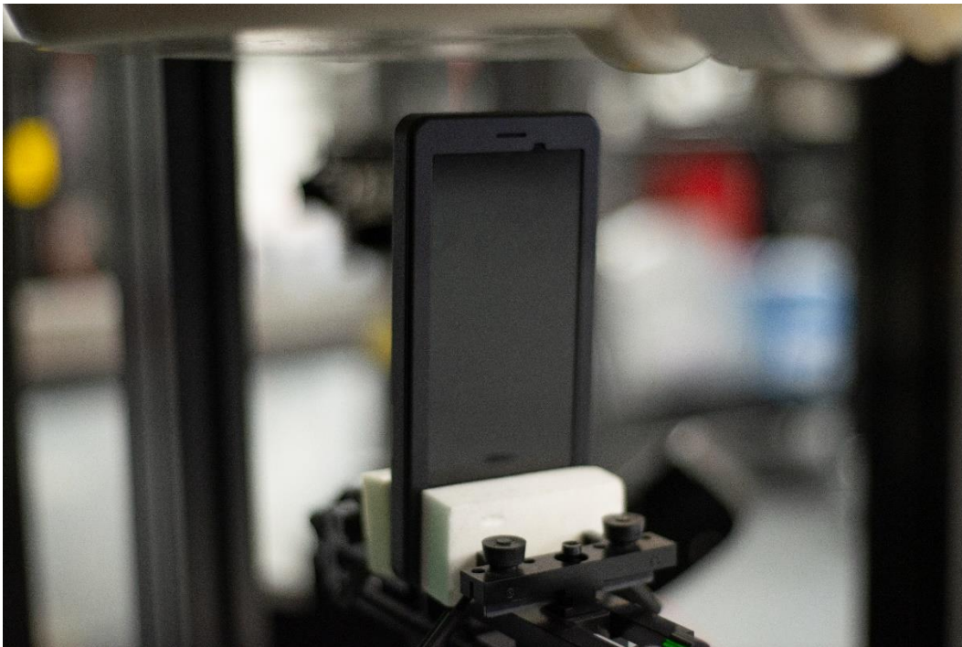
Figure F SAR Test Setup – Body – Top 25mm
