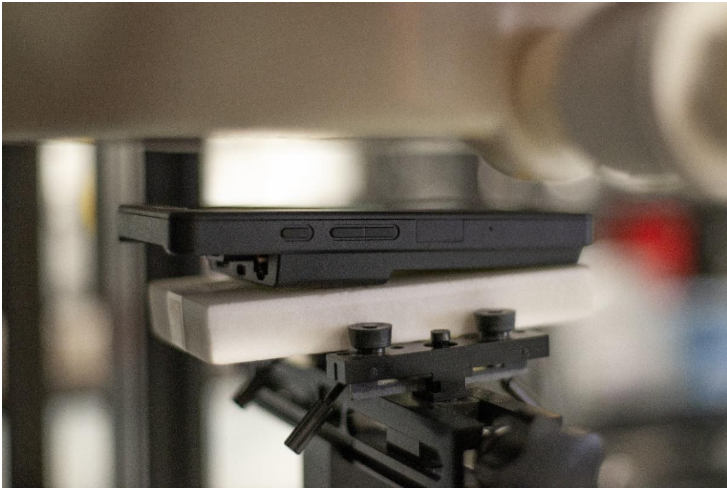
Figure D SAR Test Setup – Body – Front 25mm
