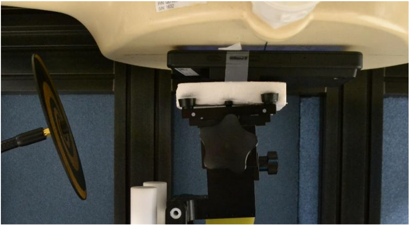
Figure C-3 SAR measurement setup
