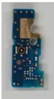
Internal Main_ANT-2-PWB (Front-side)
