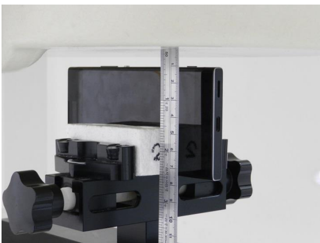
Right Side, Test Separation 10 mm
