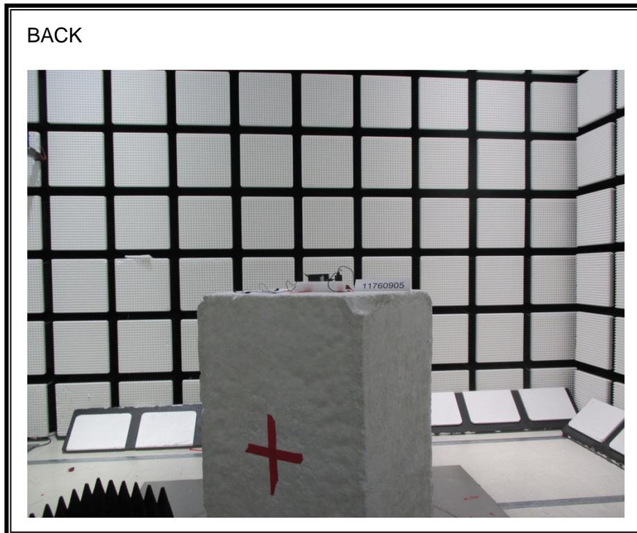
**RADIATED RF MEASUREMENT SETUP FOR PORTABLE CONFIGURATION**
