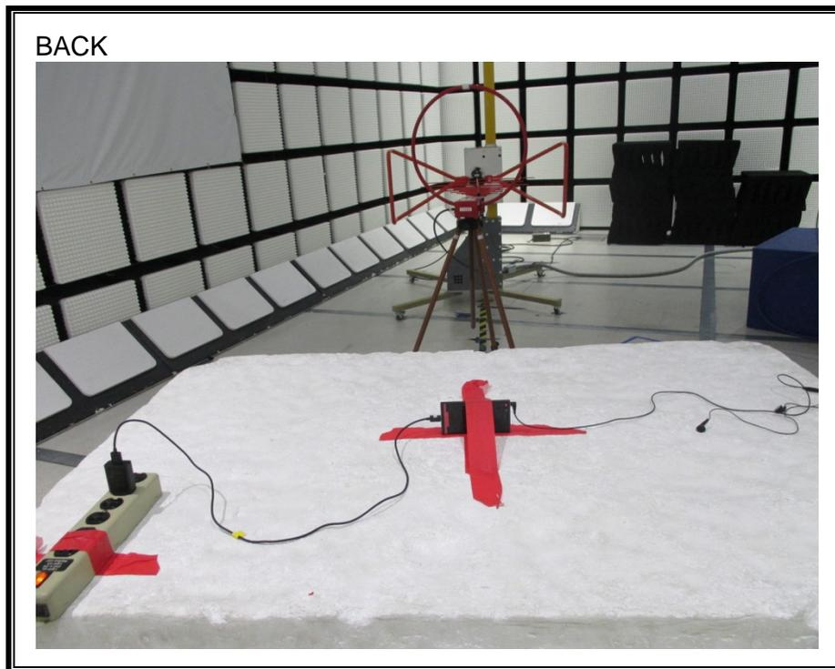
**RADIATED RF MEASUREMENT SETUP (BELOW 1 GHz)**
