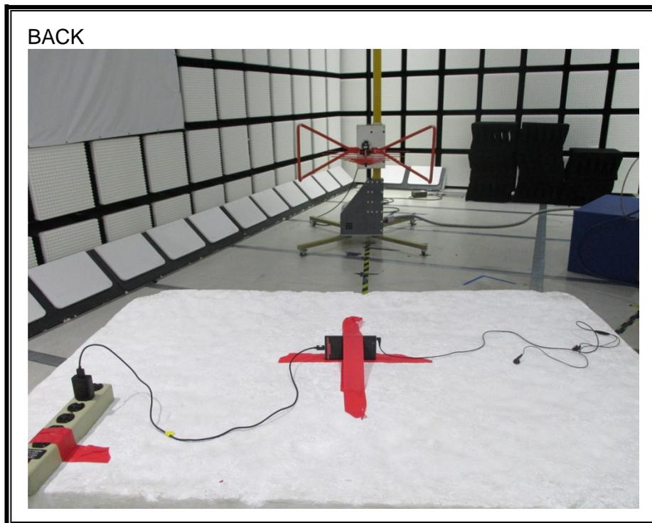
**RADIATED RF MEASUREMENT SETUP (ABOVE 1 GHz)**
