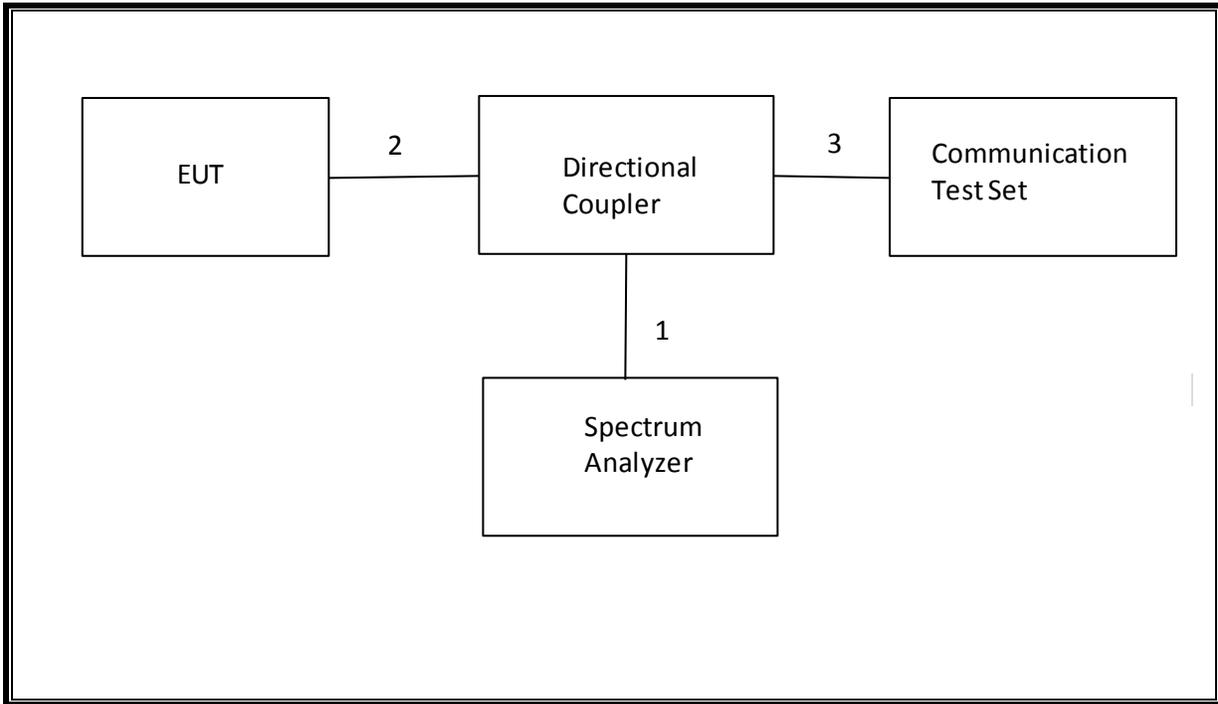
**SETUP DIAGRAM FOR TESTS (RADIATED TEST SETUP)**
