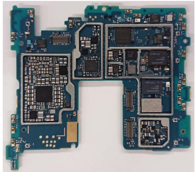
Internal PWB without Shield cases (Rear-side)
