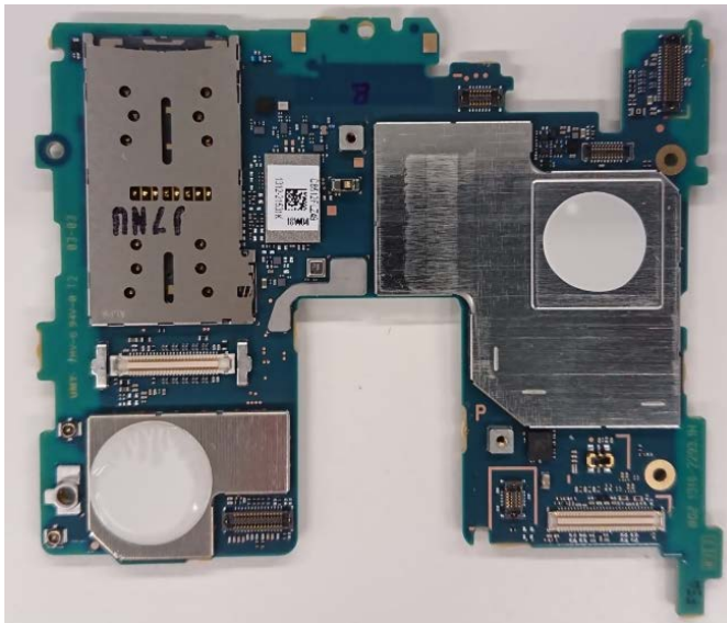
Internal PWB with Shield cases (Front-side)
