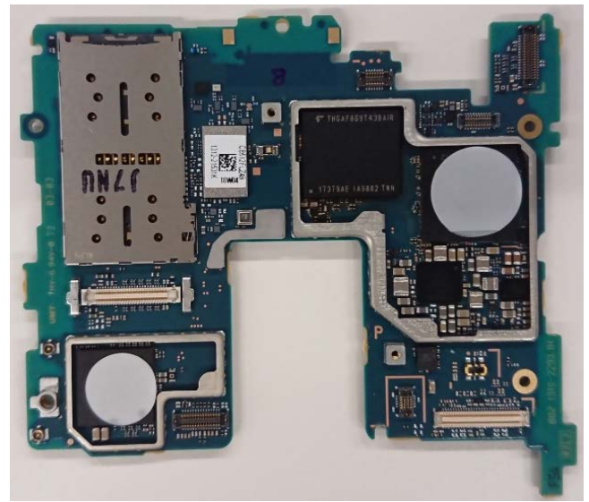
Internal PWB without Shield cases (Front-side)
