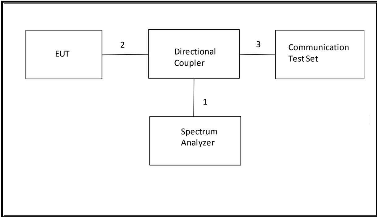
**SETUP DIAGRAM FOR TESTS (RADIATED TEST SETUP)**
