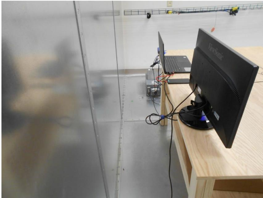
**RADIATED RF MEASUREMENT SETUP**
