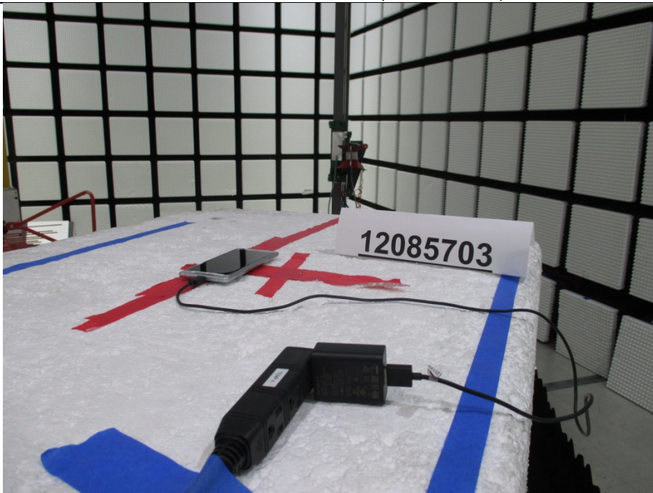
RADIATED BACK PHOTO (ABOVE 1 GHz)
