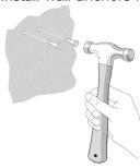
Use pan head Phillips wood screws, 3.5 x 20 mm (diameter x length, European) or #6 type screw, 1 inch long (U.S.).
