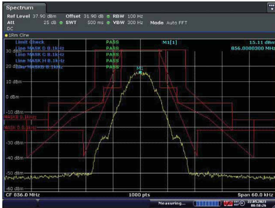
With the input signal amplitude set the AGC threshold Middle Frequency: 856.0MHz
