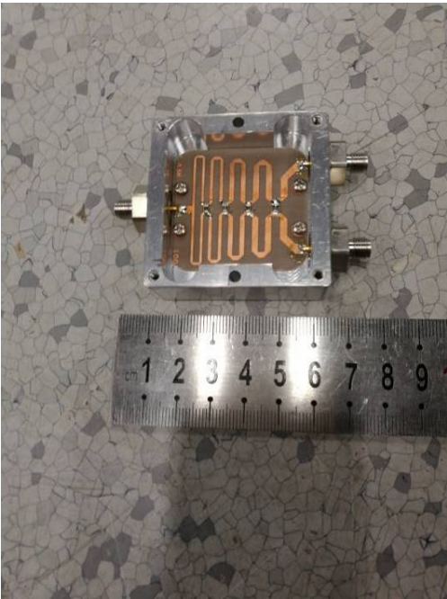
EUT – Splitter Module 3 Board View
