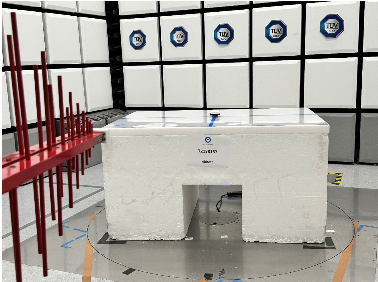
Radiated Emissions Test Setup (30MHz to 1GHz)
