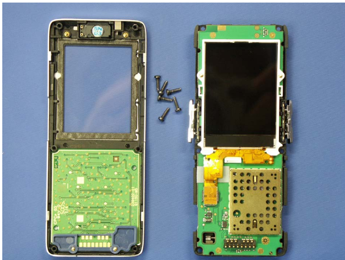
S68 PCB removed
