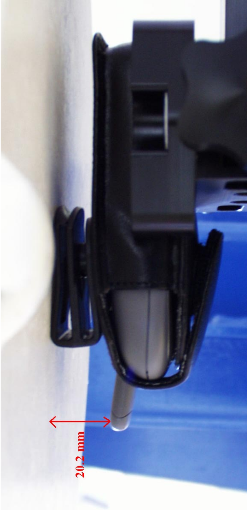
Fig. 6: Body worn configuration with leather case, display towards the ground.
