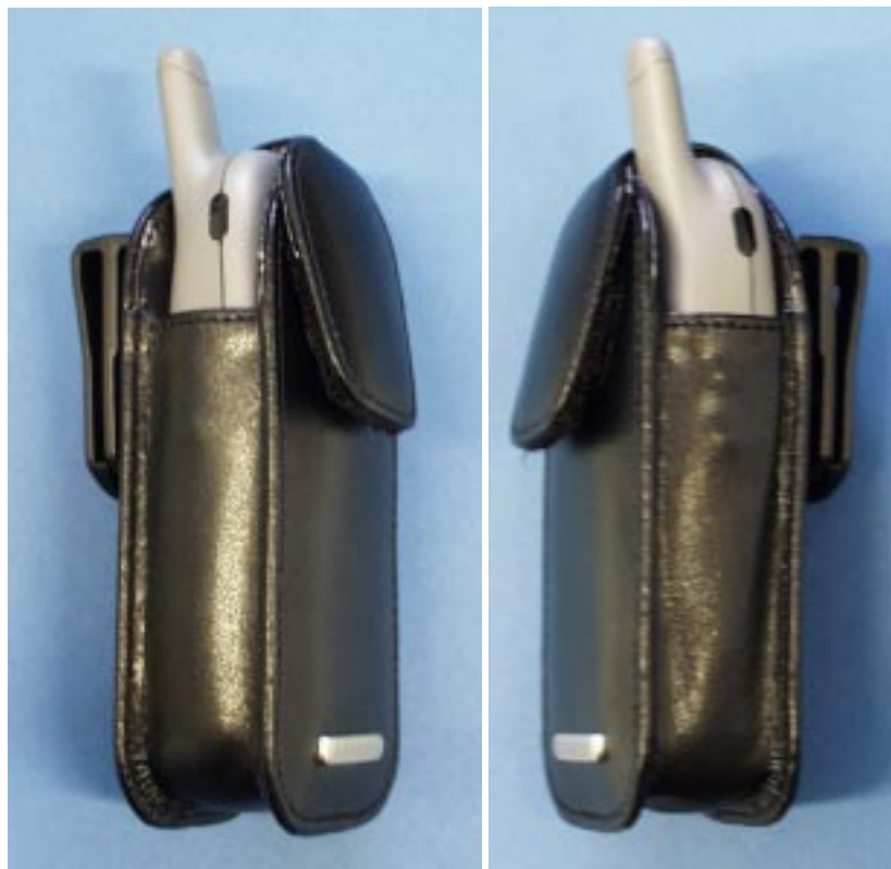
Fig. 5: Phone with leather case in the configuration: Display towards the ground (left) and Display towards the phantom (right).
