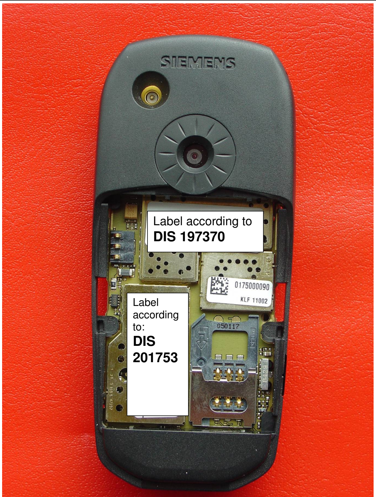
Figure 1 Placement of FCC and IMEI label on C72
