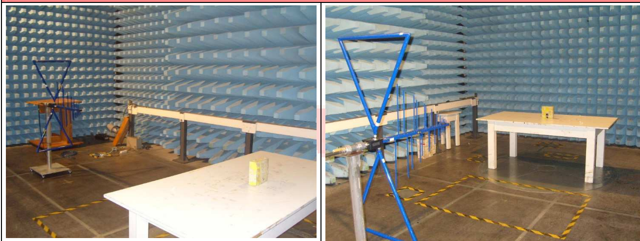
PHOTO N° 2 – RADIATED EMISSION SETUP
