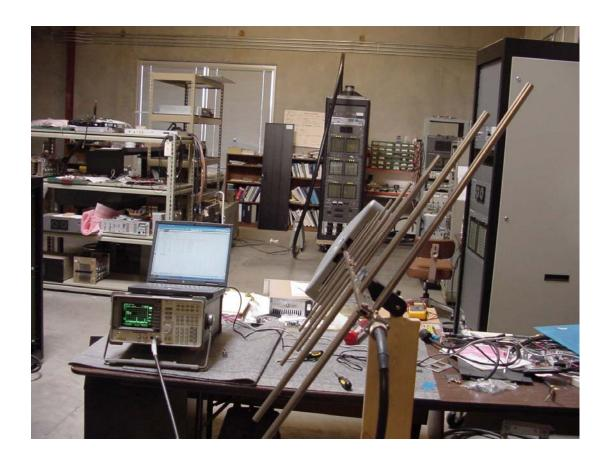
As indicated in the spreadsheet data on the following page, the worst case measurement was 72 dB at the second harmonic. (This photo above shows this particular measurement). The measurement tables for the remaining views of the transmitter are shown below.
