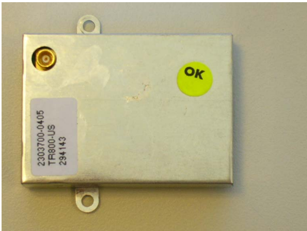
Figure 5. TR800-US. Shielded Top View.jpg
