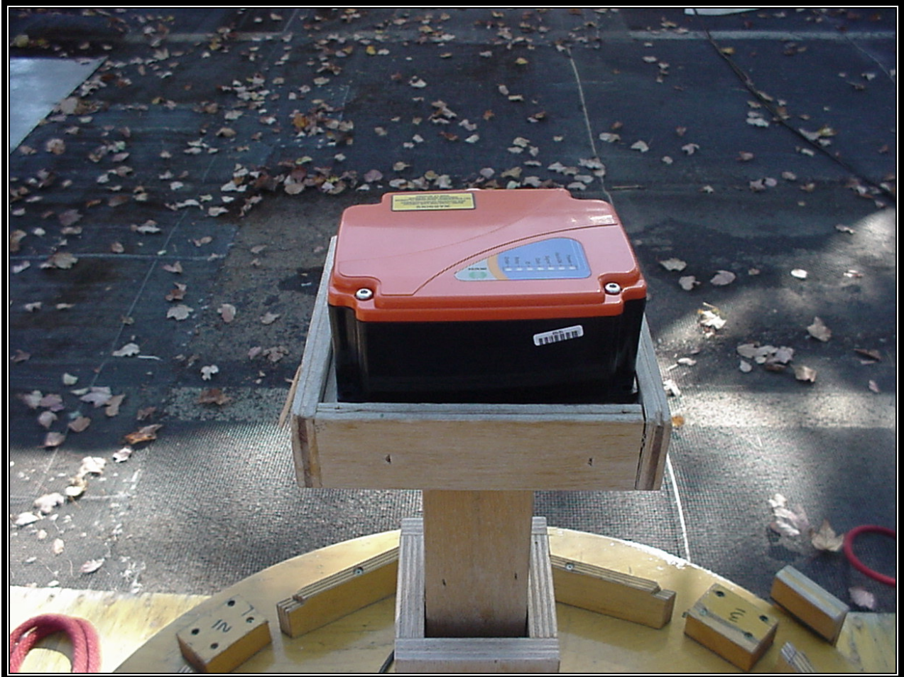
Photograph 3: Radiated Emissions - Front View
