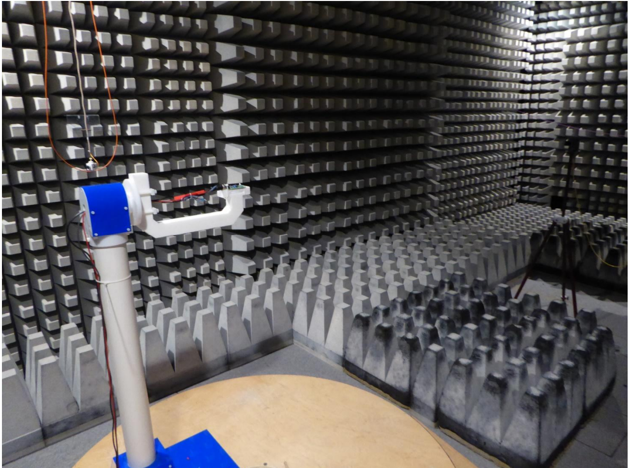
161944_TS023.jpg: Test setup fully anechoic chamber Measurement form 12 to 25/26.5 GHz
