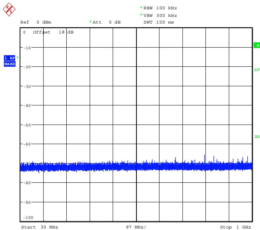
The following frequencies were found in the regarded frequency band. The results of the measurement are listed in the table below. (10.2.3.1 in [3] states that comparing to max peak is permitted).
