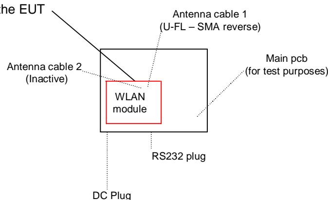
For the radiated cabinet emission tests, the worst case positioning of the EUT was investigated through measurements. The device has two possible operating positions:
