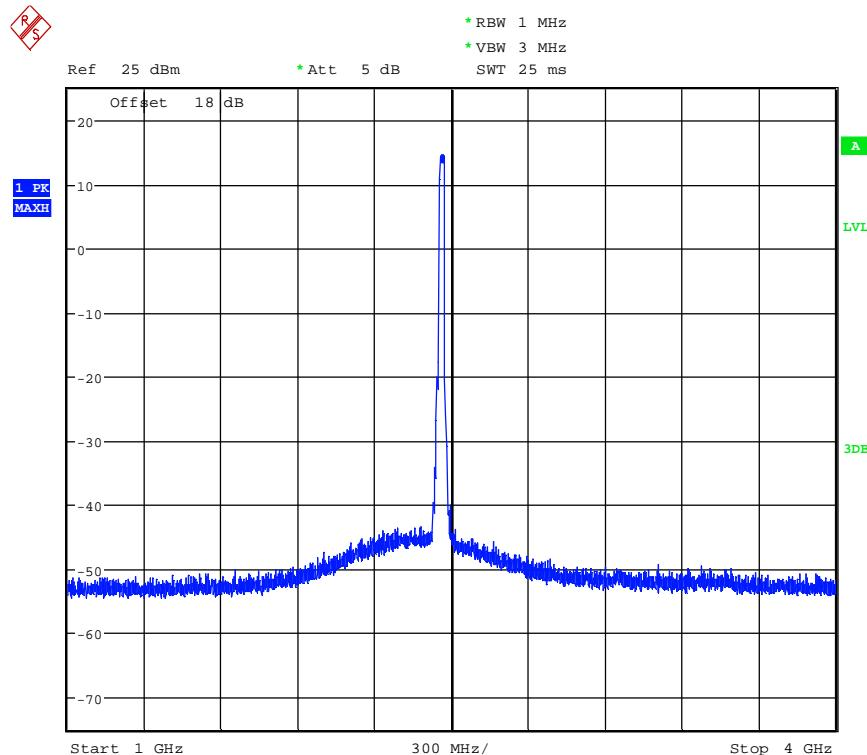
120198\_SpurEmiss4-12G\_b\_11.wmf: conducted spurious emissions (operation mode 3):
