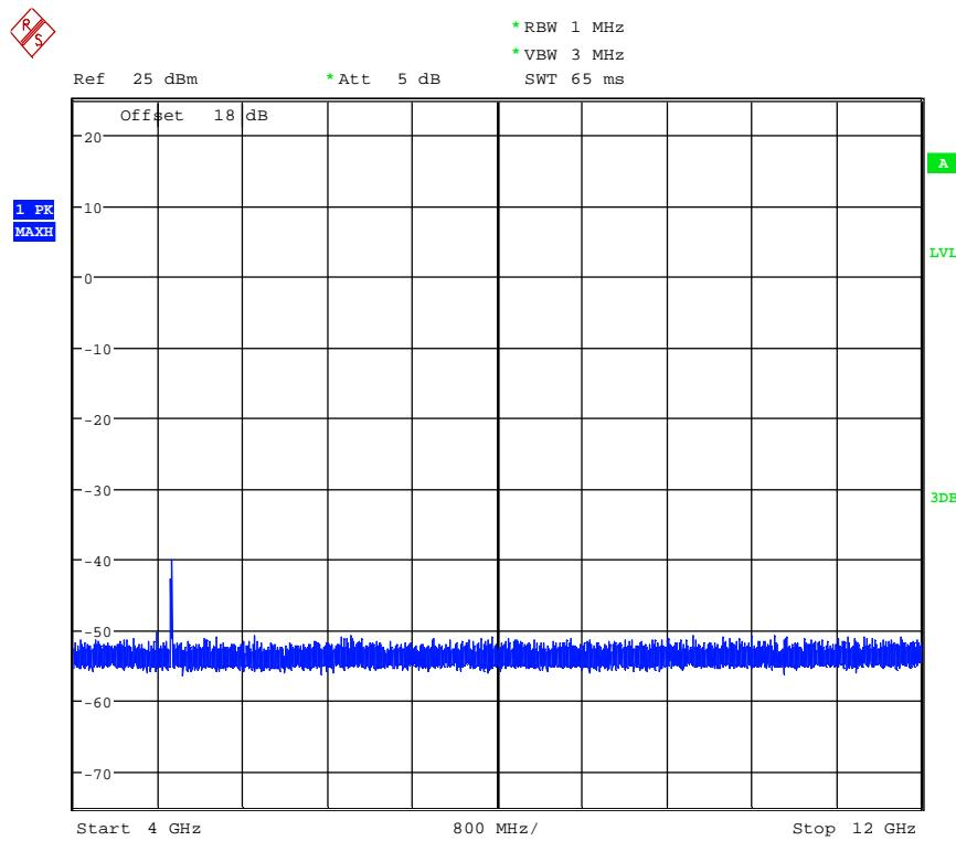
120198\_SpurEmiss12-26,5G\_b\_11.wmf: conducted spurious emissions (operation mode 3):
