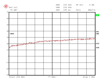
No significant frequencies above the noise floor of the system were found during the preliminary radiated emission test, so no measurements were carried out the open area test site.
