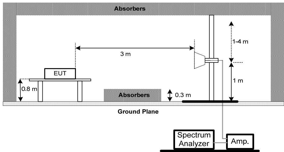
(C) For radiated emissions below 30MHz
