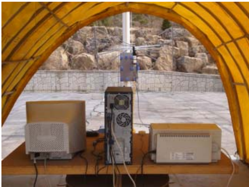
Photograph 1 : Setup for radiated Emissions
