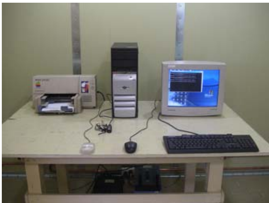
Photograph 2 : Setup for Conducted Emissions
