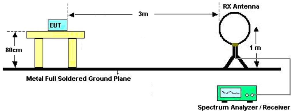
For radiated emissions from 30MHz to 1GHz
