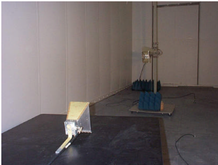
Spurious Emission Measurements, Substitution Method, Ref. Horn Antenna
