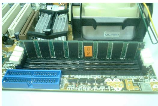
After you have set the DIMM firmly into its socket, snap the white clip holders up to lock in the DIMM.
