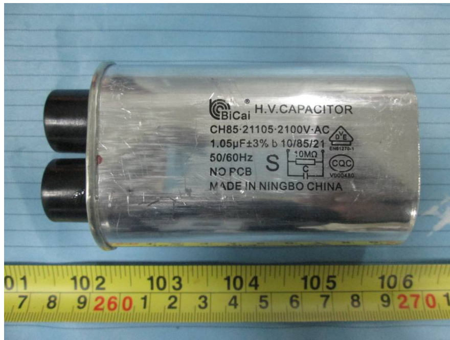
EUT – H.V. Capacitor View
