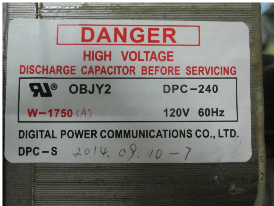
EUT – Power Transformer Label View
