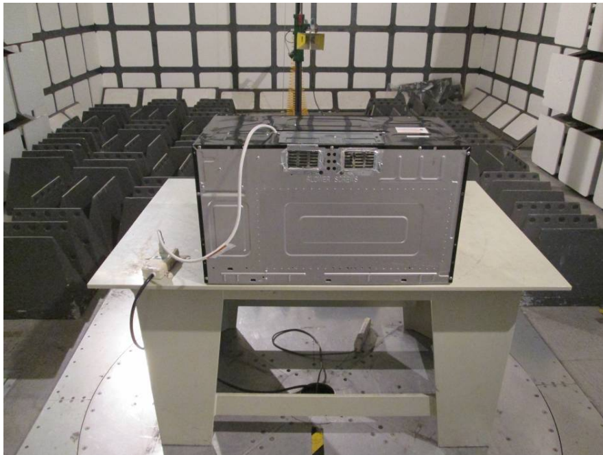
Radiated Emissions - Rear View (Above 1 GHz)
