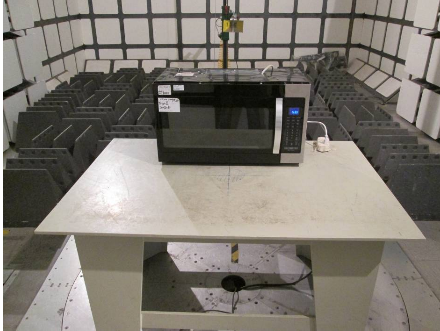
Radiated Emissions - Front View (Above 1 GHz)
