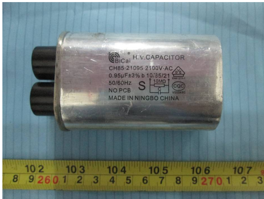
EUT – H.V. Capacitor View
