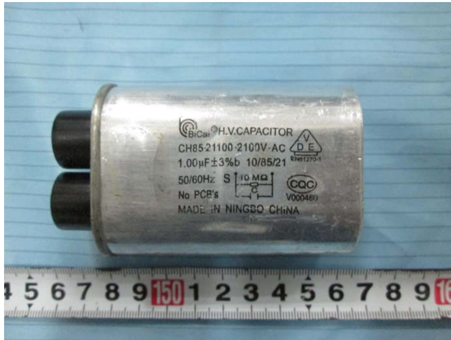
EUT – H.V. Capacitor View
