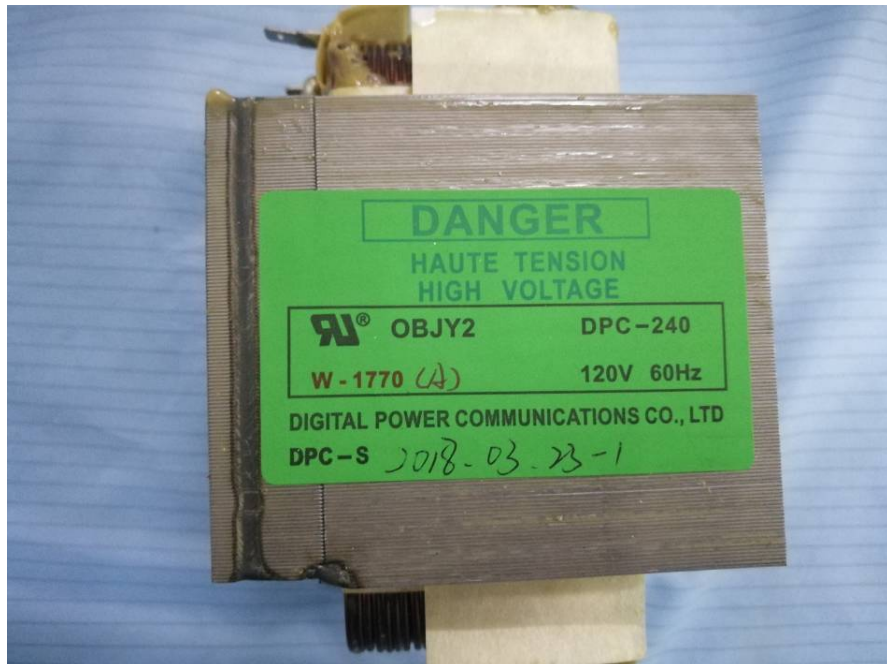
EUT – Transformer View
