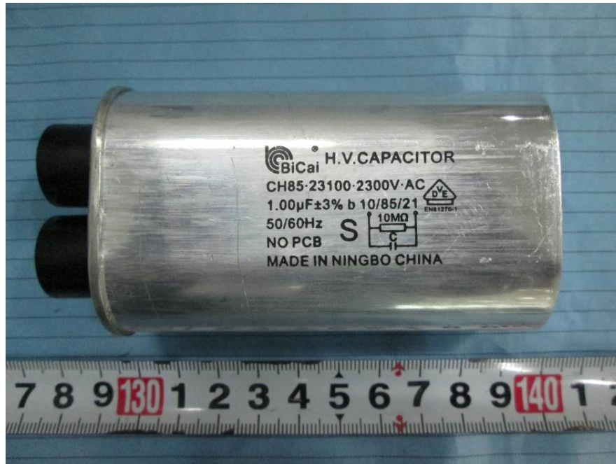
EUT – H.V. Capacitor View
