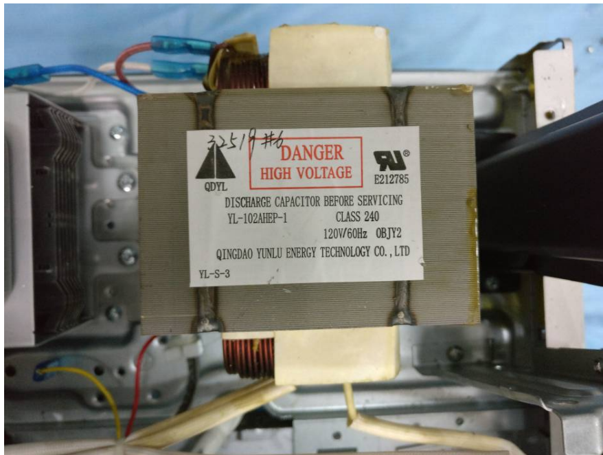
EUT – Discharge Capacitor View
