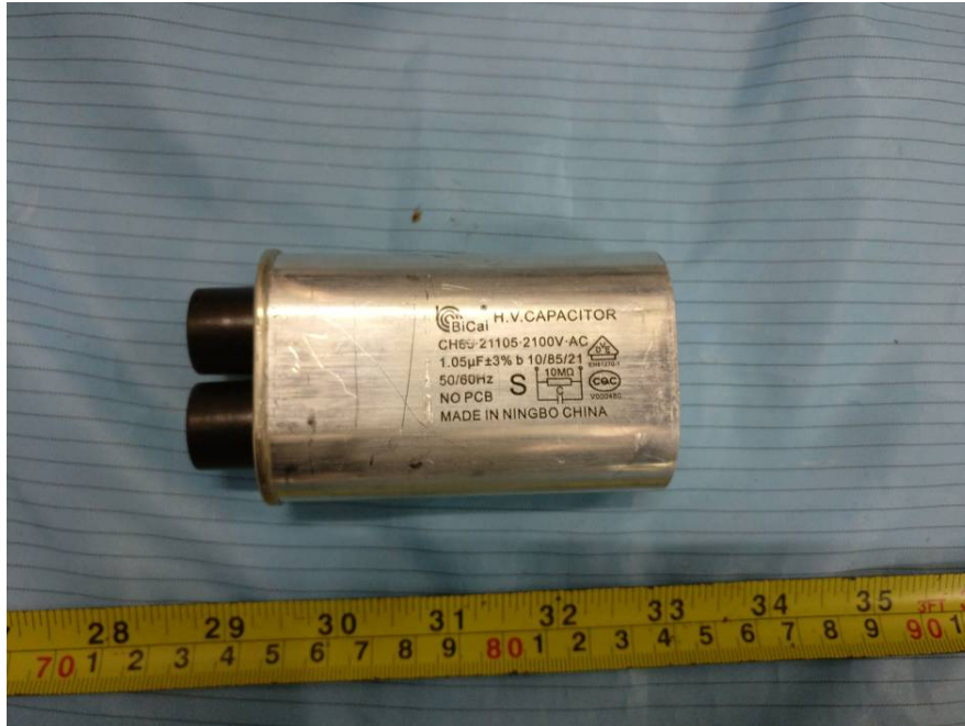
EUT – H.V. Capacitor View
