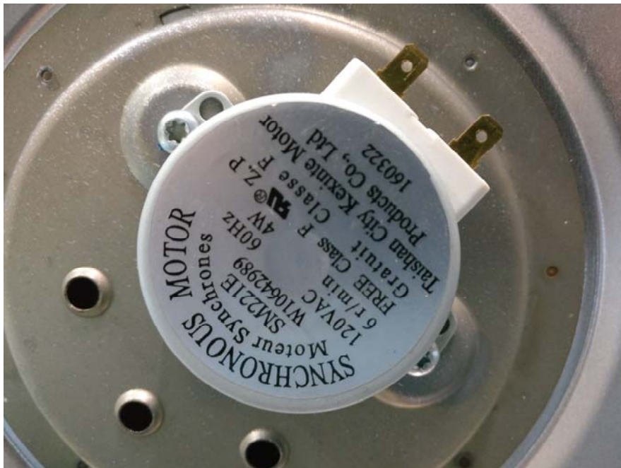
EUT – Motor Bottom Label View
