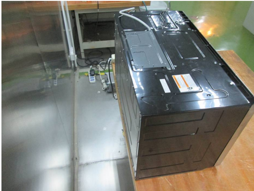
Conducted Emissions - Side View
