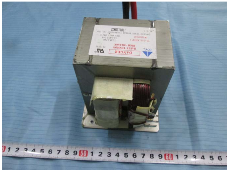
EUT – Transformer View
