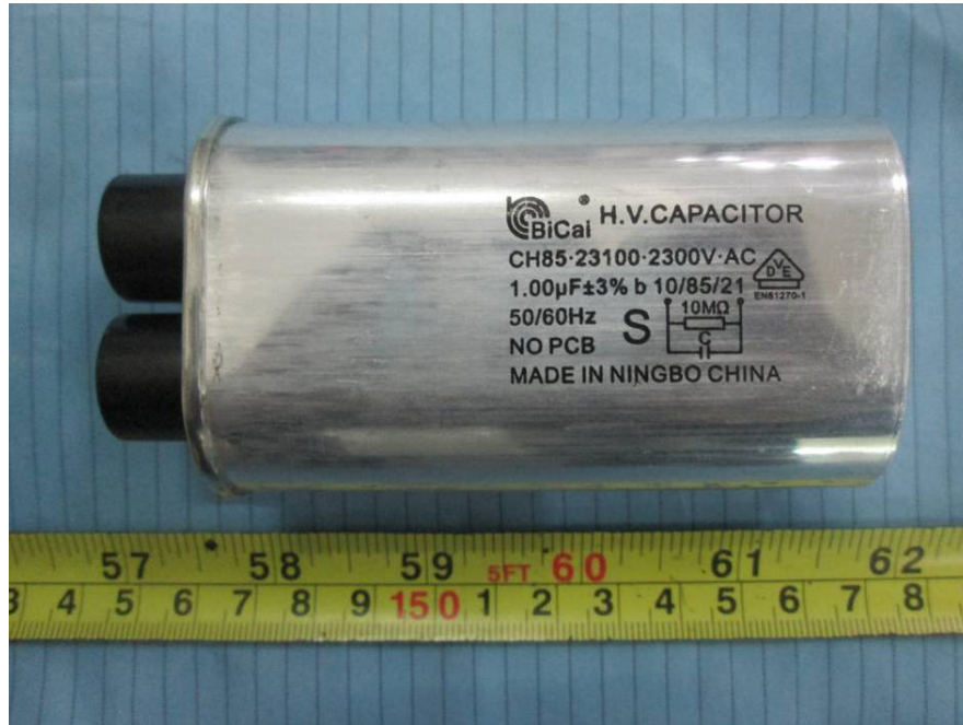
EUT –H.V. CAPACTOR View
