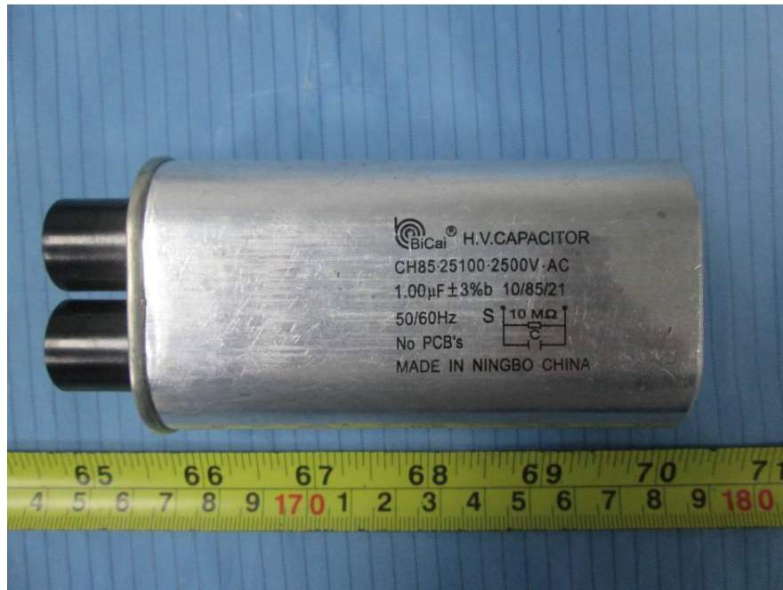
EUT – H.V. Capacitor View
