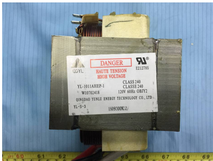
EUT – Transformer View
