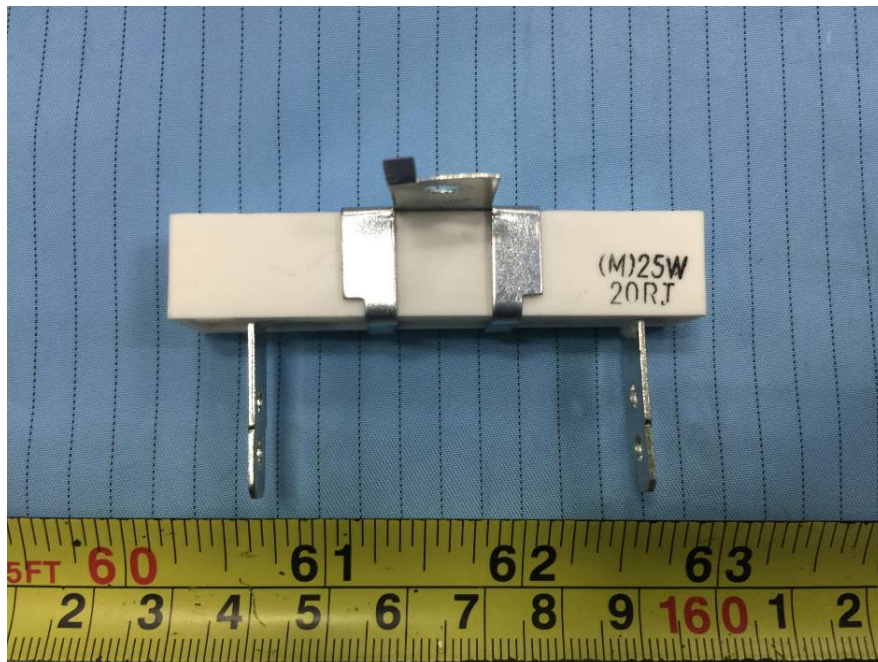
EUT – Resistor View
