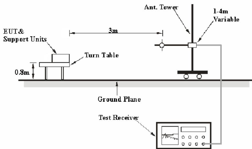
The radiated emission tests were performed in the 3 meters chamber A test site, using the setup accordance with the FCC MP - 5. The specification used was the FCC part 18 limits.
