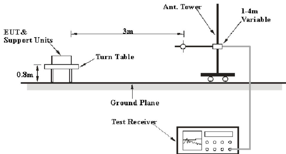
The radiated emission tests were performed in the 3 meters chamber A test site, using the setup accordance with the FCC MP - 5. The specification used was the FCC part 18 limits.
