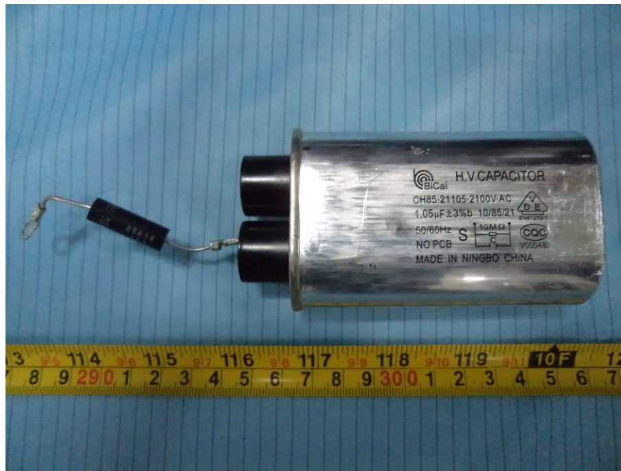
EUT – H.V. Capacitor View
