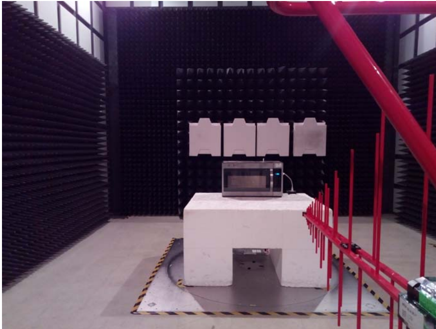
Radiated Emissions – Front View (30 MHz – 1 GHz)
