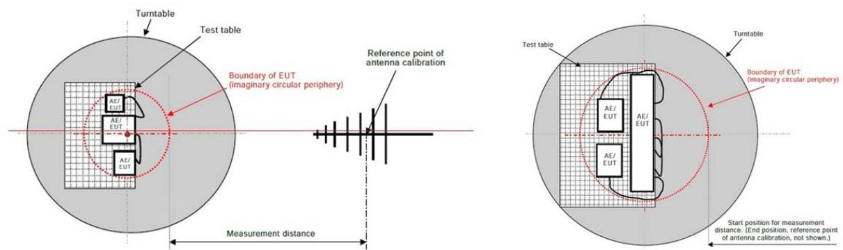
The radiated emission tests were performed in the 3 meters chamber test site, using the setup accordance with the FCC MP - 5. The specification used was the FCC part 18 limits.
