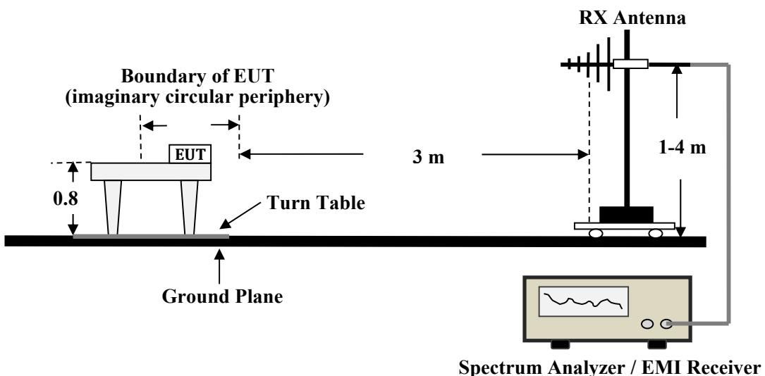
**Above 1GHz for Radiated Emissions**
