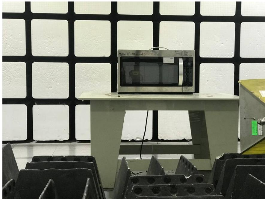
**Radiated Emissions - Rear View (Above 1 GHz)**
